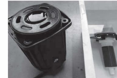
4. Put pump body in a vertical position and fill with a mild lime scale remover (like cleannning vinegar). Immerse rotor in a plastic bowl/container filled with the same lime scale remover and leave both for 24 hours. After 24h rinse off with water and re-assemble pump.
